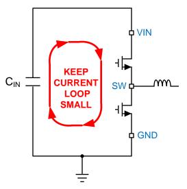
Figure 43. Current Loops with Fast Edges
