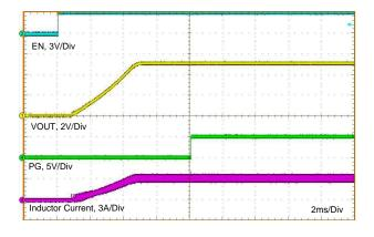
Figure 10. Typical Start-up Behavior  $V_{IN} = 12 V$ ,  $V_{OUT} = 5 V$ ,  $I_{OUT} = 3 A$
