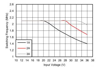
Figure 19. Switching Frequency vs Input Voltage  $V_{OUT} = 3.3 V$ ,
