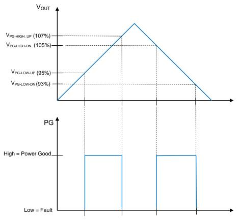
Figure 7. Static Power-Good Operation
